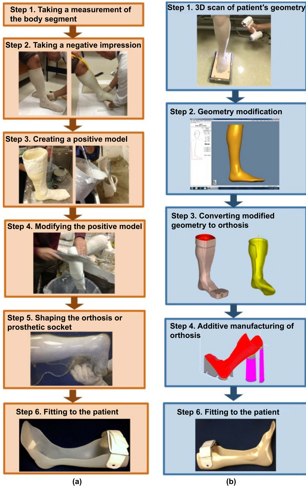
Figure 38. Traditional and AM process to fabricate AFO. Reprinted from [158], Copyright (2016), with permission from Elsevier.
